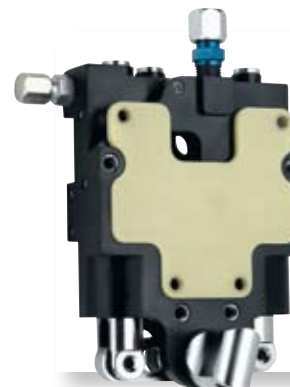
Optional isolation plates made of extremely resilient G10 improve load distribution by transferring torque directly to the mounting surface.
