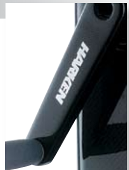
Carbon handles in place of aluminum save 1.1 kg (2.5 lb) per pedestal
