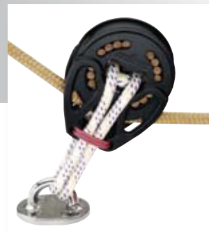
Terminating soft attachment to dead-end post allows block to be fastened to a closed bail such as a padeye
