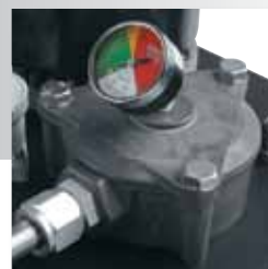
Drop-in filters and filter status gauges make maintenance fast and easy
