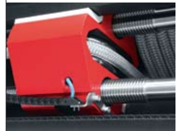
Lead screw and sheave allow line to lie smoothly on the drum—even when slack
