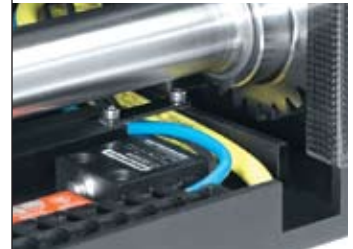
Redundant proximity switches prevent over-travel
