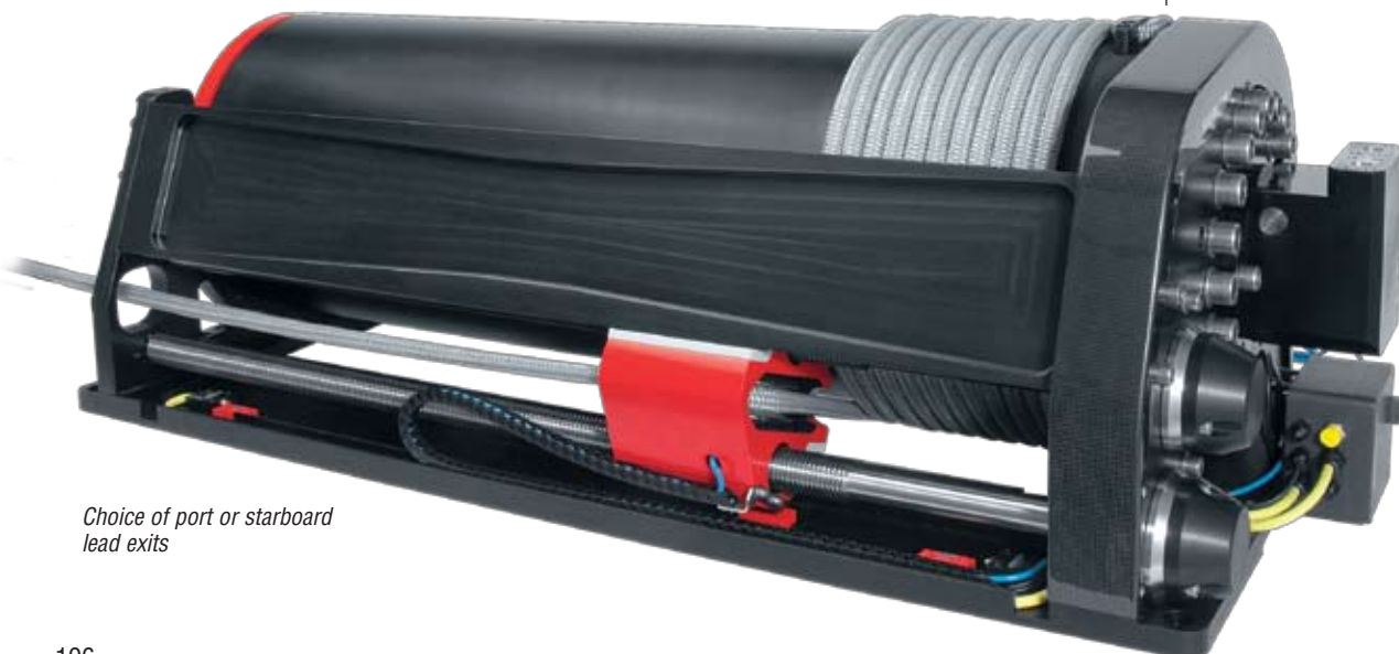
Lead screw and sheave allow line to lie smoothly on the drum—even when slack
