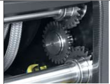
Precise gearing provides even line take-up and release
