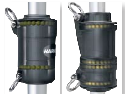
Stacked Torlon ® bearing races in the halyard swivel evenly distribute radial and thrust loads to ball bearings; foils turn freely under halyard loads
