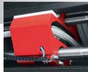
Self-lubricating feeder screw and sheave allow line to lie smoothly on the drum, even when slack.
