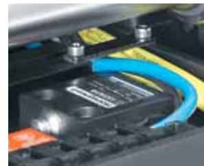
Two inner magnetic switches factory set at the feeder's stroke limits prevent over-travel. Two outer fail-safe limit switches automatically engage the brake.
