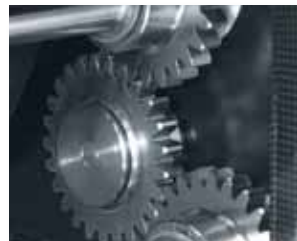
Precise gearing provides even line take-up and release.
